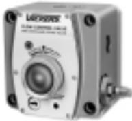
Vickers temperature and pressure compensated flow controls allow precise volumetric control. These valves are available with (bypass type) or without (restrictor type) integral relief valves and are suitable for pressures up to 250 bar (3600 psi).
