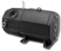
The Vickers Integrated Motor Pump is a unique combination of a conventional AC induction motor cooled with system hydraulic oil and Vickers hydraulic pump, either fixed vane pump or variable piston type, housed in a special sound reduction enclosure. This combination provides an exceptionally quiet and small pumping package for any industrial application requiring up to 125 horsepower (92 kilowatts) of continuous hydraulic power.
