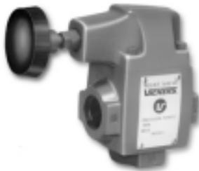
Small, easily installed remote pressure control valves make it possible to control a balanced piston pressure relief valve from a more convenient location. Available pressure ranges for the CGR-02 valve are from 4,5 to 70 bar (65 to 1000 psi), from 4,5 to 140 bar (65 to 2000 psi), and from 4,5 to 210 bar (65 to 3000 psi).
