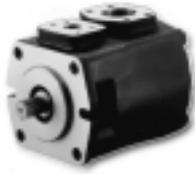
Vickers offers an extensive line of fixed displacement single pumps with displacements from 3,3 to 215 cm<sup>3</sup>/r (.20 to 13.12 in<sup>3</sup>/r); continuous pressures to 280 bar (4000 psi); speeds to 7000 r/min. V10 and V20 models can be provided with integral valving to limit flow to the operating system, to limit maximum system pressure, and to divide flow between two circuits. VTM42 pumps are for power steering applications. VQ, VMQ and VPF models are available with thru-drives.
