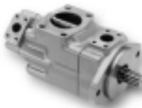
Vickers extensive line of fixed displacement double pumps offers: displacements from 22,8 to 390 cm<sup>3</sup>/r (1.39 to 23.78 in<sup>3</sup>/r); continuous pressures to 280 bar (4000 psi); speeds to 3000 r/min. V2010 and V2020 models can be provided with integral valving to limit flow to the operating system, to limit maximum system pressure, and to divide flow between two circuits. VQ models are available with thru-drives.
