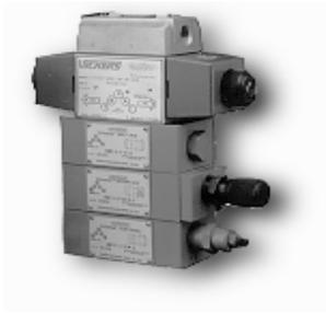
SystemStak™ valves make compact hydraulic systems in which modular valves are “sandwich” mounted between a directional control valve and a standard mounting surface. All circuit flow paths are contained within the control valve and modules. With their cartridge design they provide a compact hydraulic circuit at a reduced cost with the elimination of interconnecting piping.
