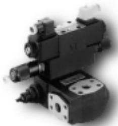
Flange mounted valves mount directly to the pump flange and reduce potential leak points for superior leak resistance. Three different valves are available: relief, unloading and check. Pilot design minimizes response time and cracking flow which allows for high pressure stability and increased system productivity.
