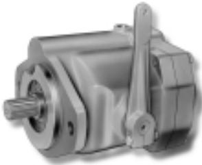
Vickers variable displacement piston motors offer: two displacements of 19,5 and 21,1 cm<sup>3</sup>/r (0.64 and 1.29 in<sup>3</sup>/r); flows from 19,0 to 68,1 l/min (5.0 to 18.0 USgpm); speed ranges dependent on input flow and displacement control with a range of 4:1 to 12:1. MVB5 and MVB10 motors will operate at speeds as low as 50 rpm with appropriate circuit and application considerations.
