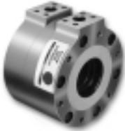
Vickers high torque, low speed vane motors offer: displacements from 24 to 754 cm<sup>3</sup>/r (393 to 12356 in<sup>3</sup>/r); pressures to 280 bar (4000 psi); speeds to 400 r/min; a choice of 14 single torque, single displacement models or 12 multi-torque, multi-displacement models.
