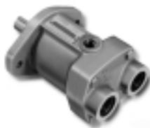
PFB fixed displacement piston pumps are available in four geometric displacements: 10,5; 21,1; 42,8 and 94,4 cm<sup>3</sup>/rev (0.64, 2.61 and 5.76 in<sup>3</sup>/rev). Depending upon displacement and type of fluid used, maximum speeds are from 1200 to 3600 r/min, and maximum operating pressures are from 69 to 207 bar (1000 to 3000 psi). Foot mountings are available for all models.
