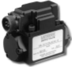
Vickers servovalves are two-stage, four-way, flapper nozzle valves that provide system closed loop control with exact positional accuracy, repeatable velocity profiles and predictable force or torque regulations.
